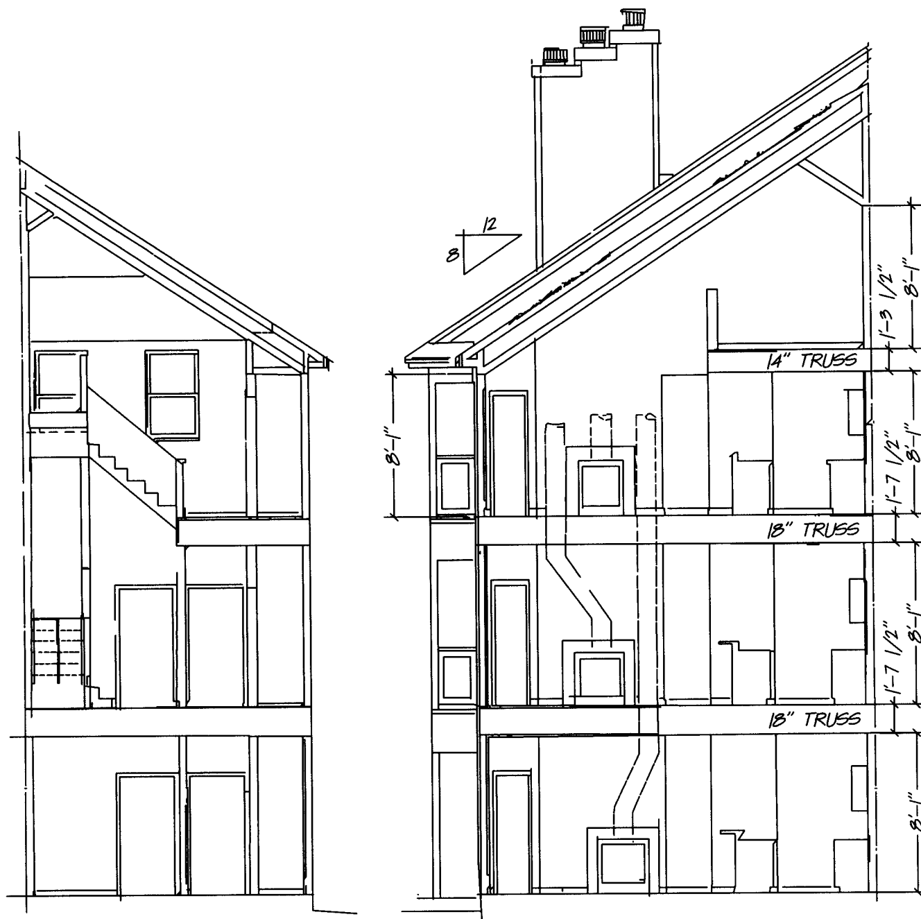
SECTIONS THROUGH STAIRWELL & LIVING ROOM / KITCHEN
